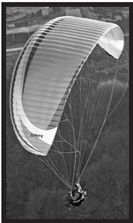
The **ZEPHYR** has a brake of medium weight resistance (from 1.5 to 3 kg of force) for the majority of manoeuvres. To reach the stall (never recommended on any type of paraglider), requires more than 9kg.
