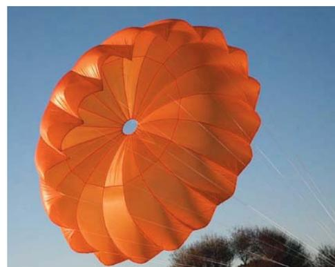
*A PDA specific design with a flatter canopy to obtain a bigger projected surface and improve the performance during descent.*
