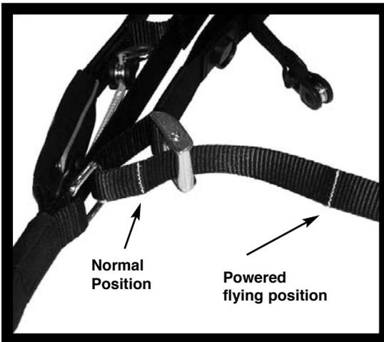
the trimmers are set to compensate for the pitching back effect caused by the push of the motor, bringing the wing into a more overhead position and giving increased speed and performance. Of course, caution should always be used when low down and one should always fly with the trimmers in the "normal" trim position in turbulence and when near the ground.
