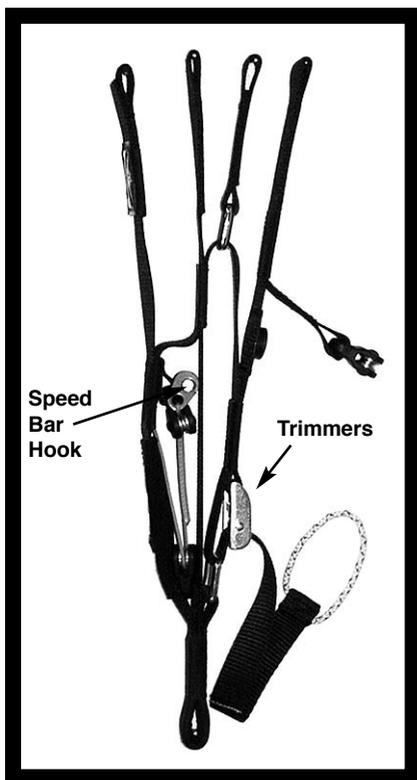
The risers are shorter than usual (42cm), to allow for the different flying position and help minimise the effects of the chassis of the engine.
