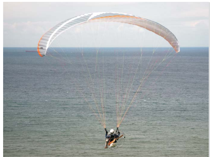
Which size Evo to choose is affected by the power of your engine and flight altitude.
