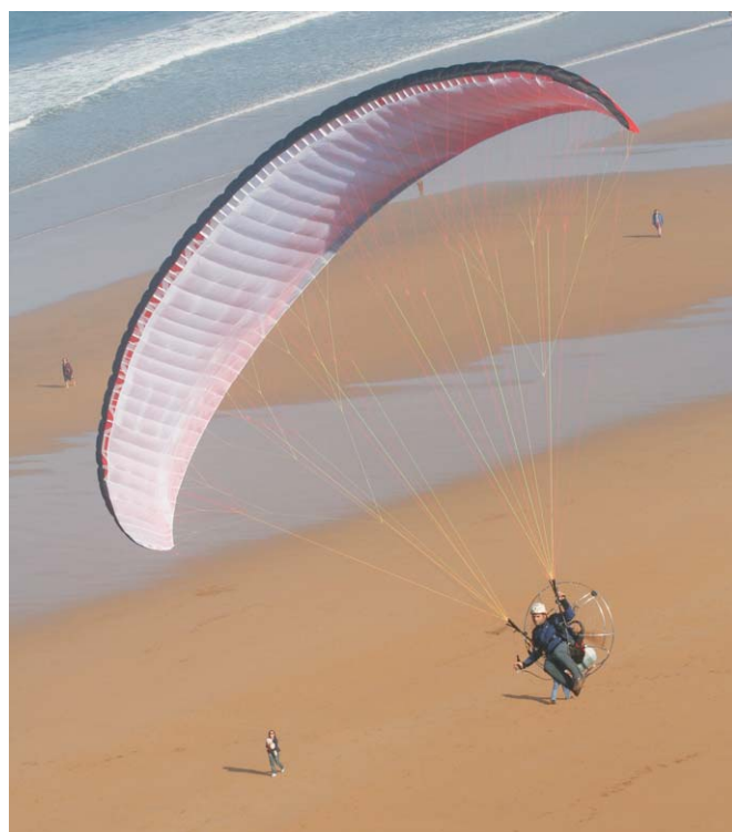
The leading edge equipped with the S.A.S. is easy to see in this photo.
